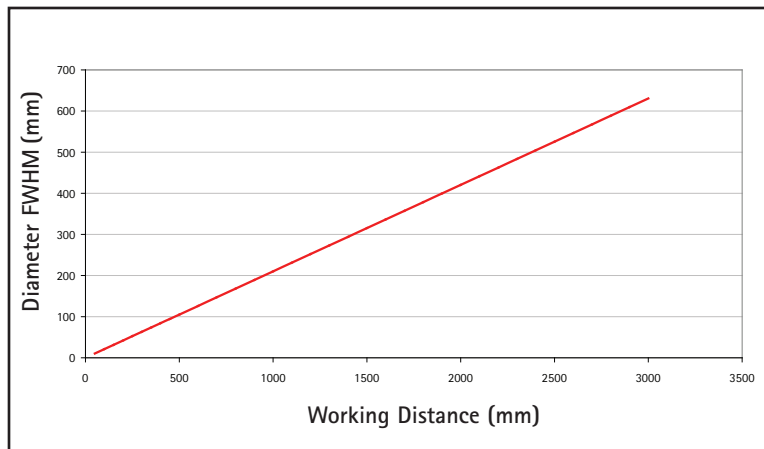
Figure 2 - Diameter of field of illumination vs. working distance for all wavelengths.
